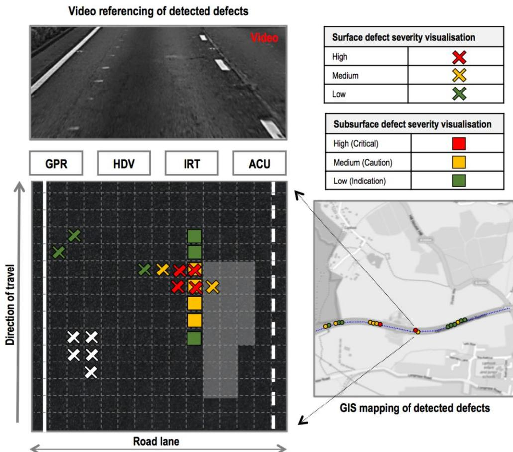
Figure 8. RPB HealTec system: decision-support output
